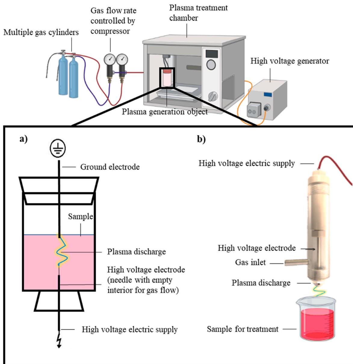
Fig. 2. Schematic set-up of atmospheric a) cold plasma discharge system (CPDS); b) cold plasma jet system (CPJS).
