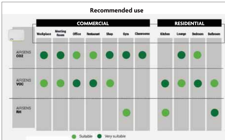
Chart shows the recommended usage values of the Airsens fan range in various commercial and residential settings.
