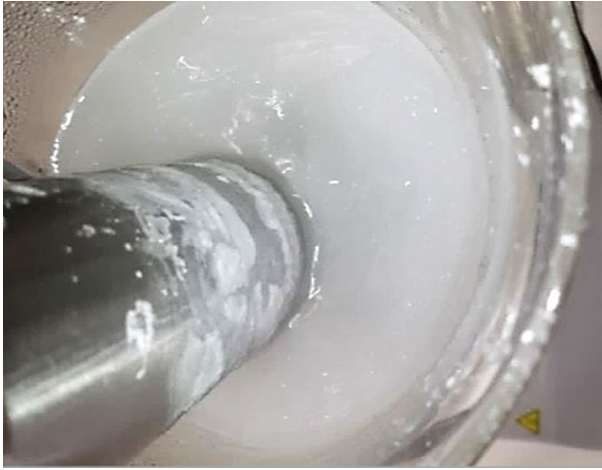
Fig. 8 Visible incrustation on an immersible probe during crystallization. The experiment included gradual decrease of temperature during which there was continuous stirring in an open container and a normally occurring evaporation. A ‘crust’ due to the dissolved chemical formed on the stainless steel body
