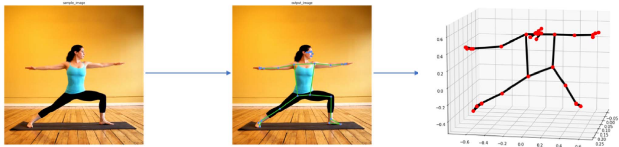
Fig. 3: 3D Landmarks data on warrior pose using BlazePose model
