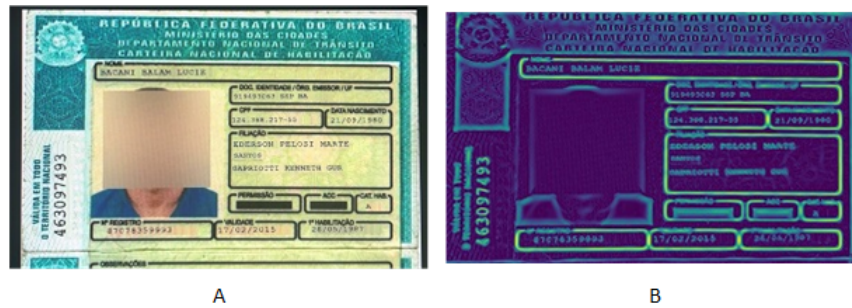
Fig. 3. Artifacts added to the BID data set to assist with document segmentation result in features extracted by the Meijering filter that would not exist otherwise. Image A is an example where the authors added bold borders around the biographic textual fields. Image B, obtained by applying the Meijering filter to image A, clearly shows that the artifacts added in Image A result in distinct bright lines where the bold borders were introduced.
