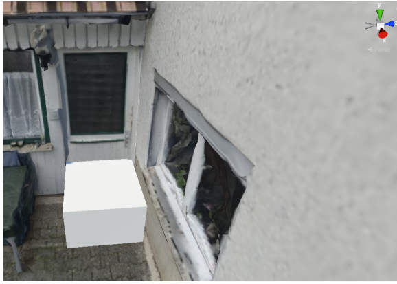
Fig. 3. A 3D Scanned scene containing a door, scaled to the 0.8m reference object (pictured in white).
