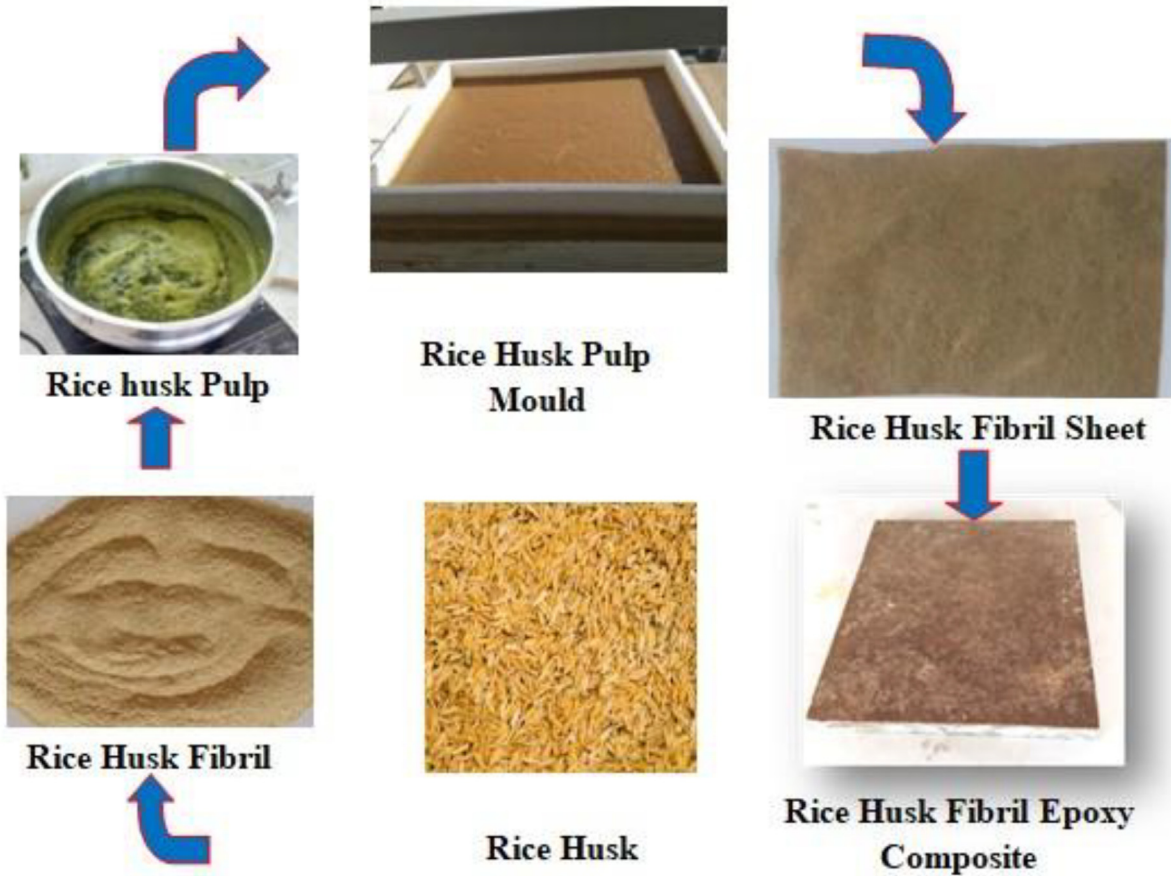
Fig. 1 – A graphic view of fabrication of rice husk fibril reinforced epoxy composites.
