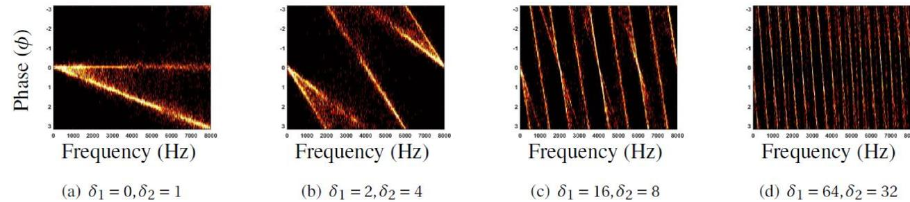
Figure 1: The delays,  $\delta_j$  are in samples. The slanting lines are observed for real speech utterances, where each line corresponds to a source,  $s_j[n]$ . The larger the delay, the more often the lines get phase wrapped. They indicate the energy concentration of a particular phase bin as a function of frequency.
