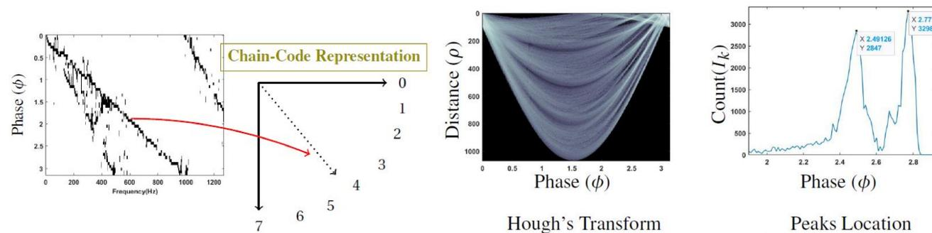
Figure 3: Two figures on LHS: Each code in 0 – 7 corresponds to a particular direction. RHS figure most two most prominent peaks are observed at  $\phi = 2.49$  and  $2.77$  rads. These corresponds to two accumulator cells getting two highest votes.
