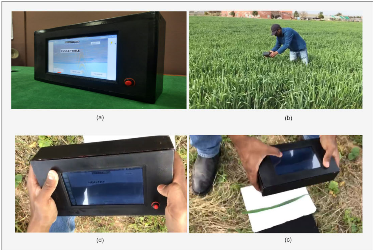
FIGURE 9. Wheat rust disease detection device testing (a) Testing in the Lab (b) Image capturing in wheat fields, (c) Testing device with constant white background (d) Result of (c).
