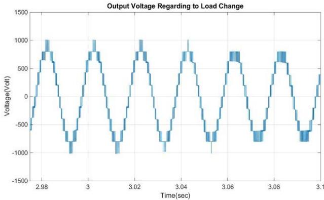
Fig. 6. Inverter Output Voltage with load change at  $t=3s$
