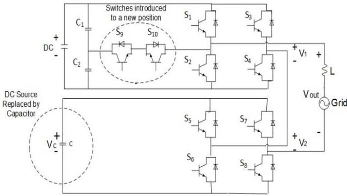
Fig. 1. Proposed Grid-tied Multi-level Topology
