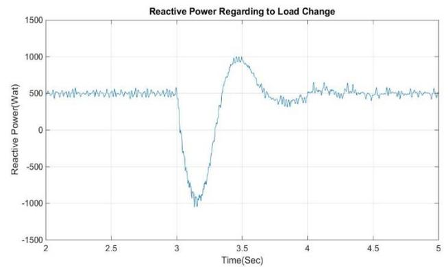
Fig. 10. Reactive Power to the Grid (Fixed Reactive Power Reference)
