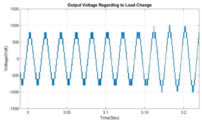
Fig. 11. Inverter Output Voltage with load change at  $t=3s$
