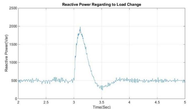
Fig. 5. Reactive Power to the Grid (Reference Changes from 10kW to 7kW)
