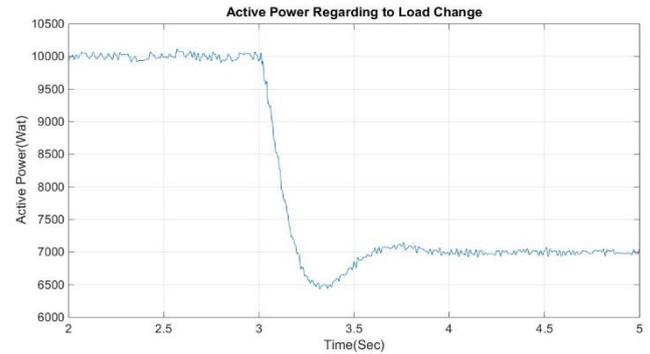
Fig. 4. Active Power to the Grid (Reference Changes from 10kW to 7kW)
