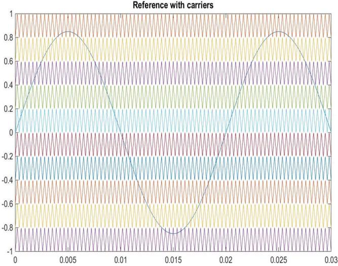
Fig. 2. Reference signal with multi-carrier level shifted PWM
