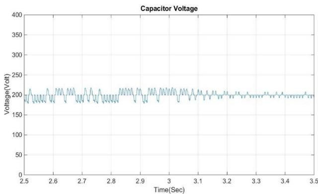
Fig. 8. Capacitor Voltage (Reference Changes from 10kW to 7kW)
