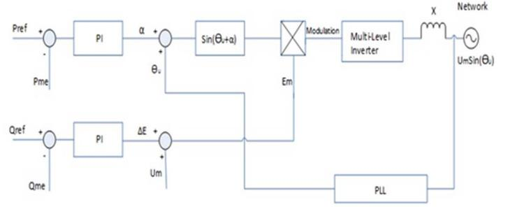
Fig. 3. Control structure for a single phase grid connected MMC
