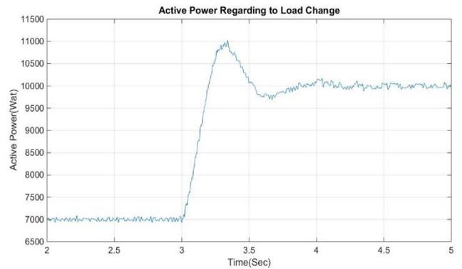
Fig. 9. Active Power to the Grid (Reference Changes from 7kW to 10kW)
