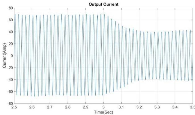
Fig. 7. Inverter Output Current (Reference Changes from 10kW to 7kW)
