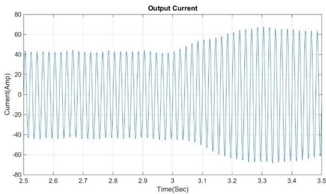
Fig. 12. Inverter Output Current (Reference Changes from 7kW to 10kW)
