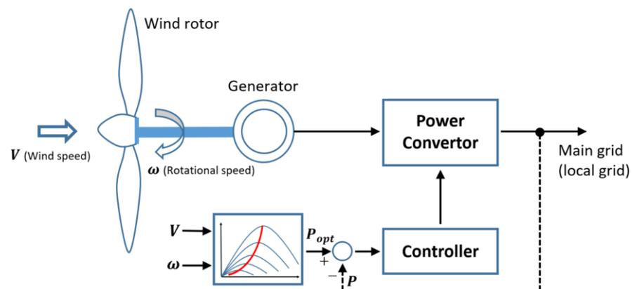
**Figure 12.** Control strategy of a wind turbine system.
