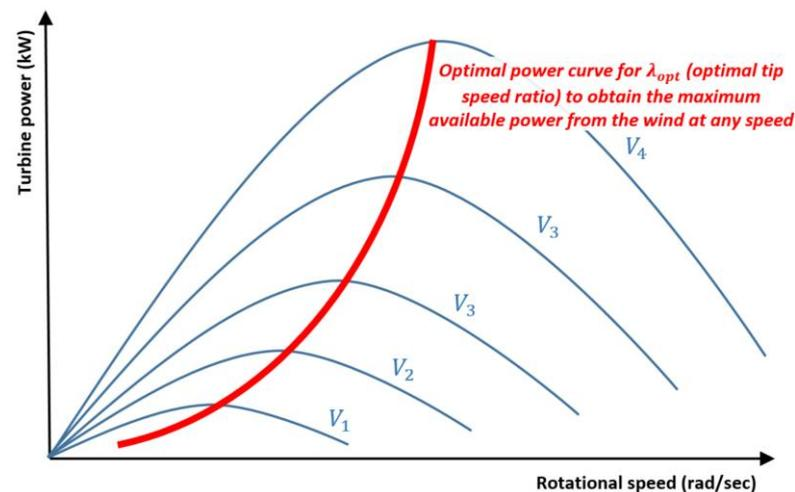
**Figure 11.** Wind rotor power vs. rotational speed for different wind speeds.
