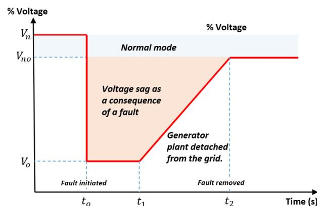
**Figure 8.** Generic fault ride-through capability curve.
