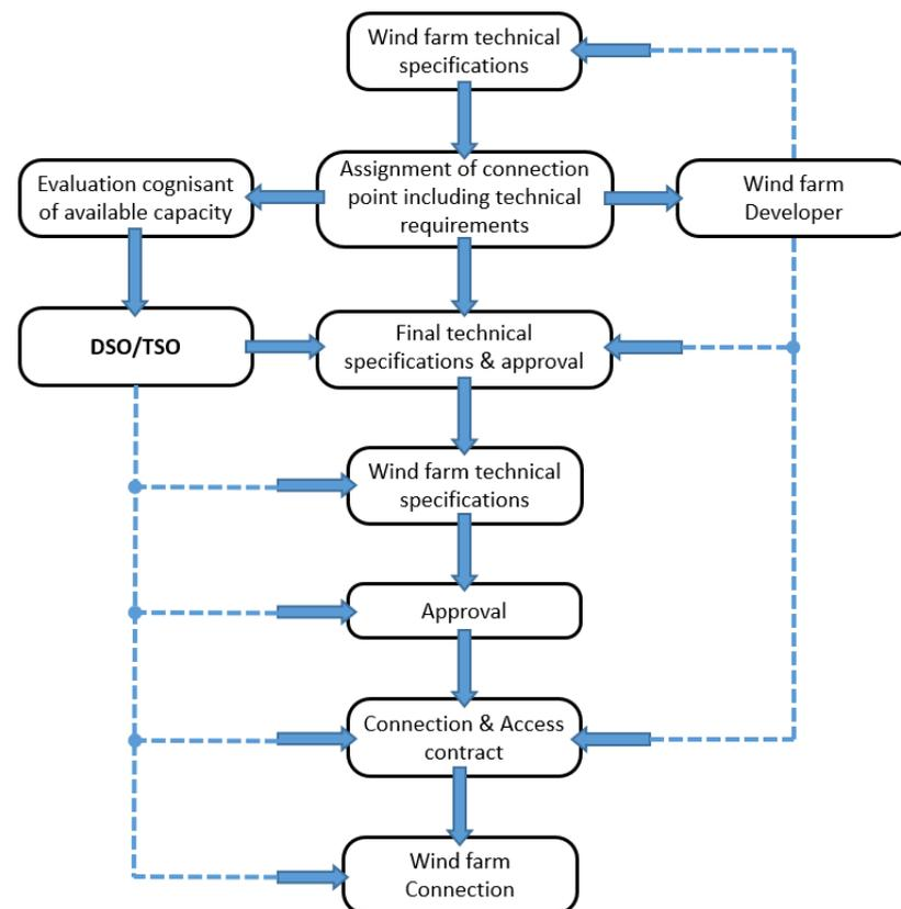
**Figure 9.** General connection procedure for wind power plants.
