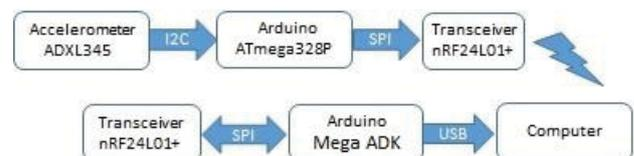
Fig. 3 Wireless MMG sensor
