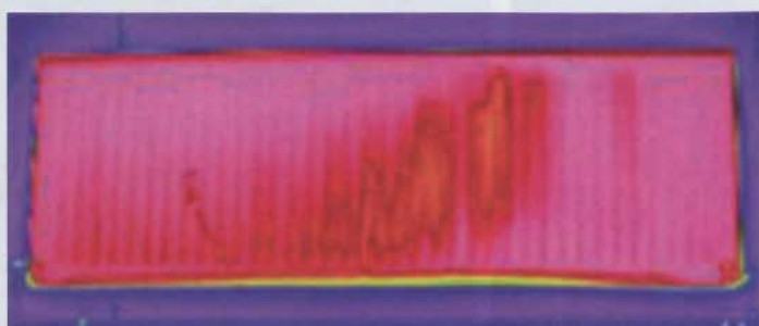
Above — Thermal image of a radiator prior to Sentinel chemical water treatment; Below — the same radiator after treatment
