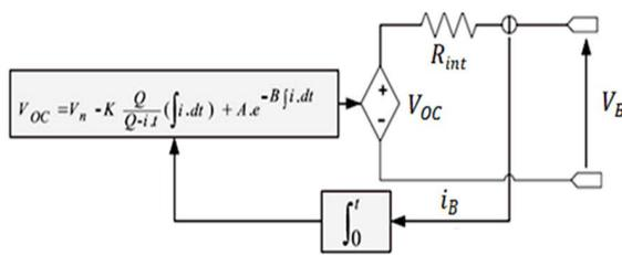
FIGURE 3. The battery electrical circuit module.
