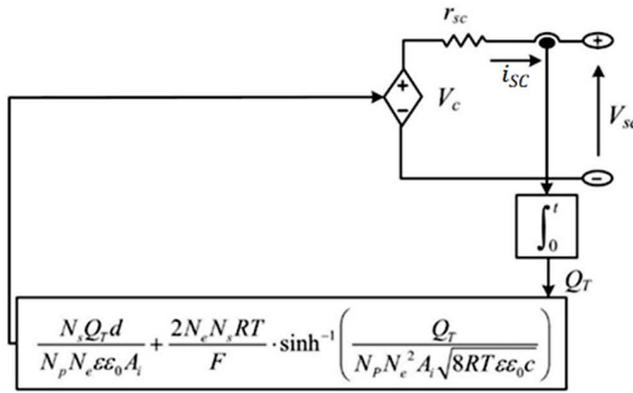
FIGURE 2. The SC equivalent circuit module.
