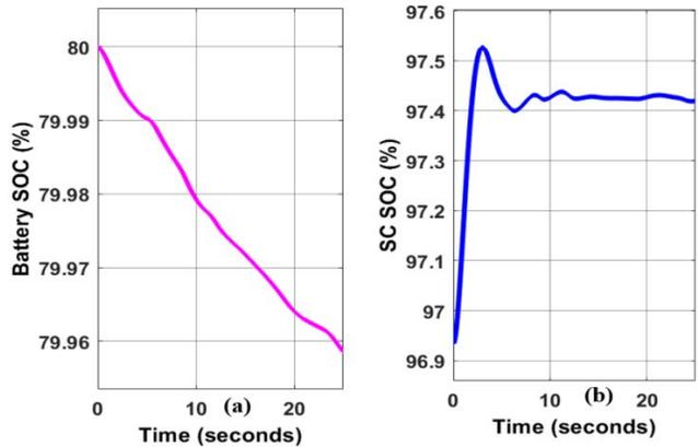
FIGURE 9. The SOC simulation results (a) the SOC of the battery (b) the SOC of the SC.
