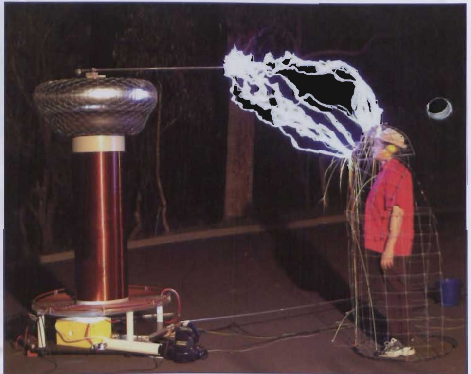
Figure 2 — The Faraday Cage Experiment. (Image courtesy of Tesladownunder.com)
