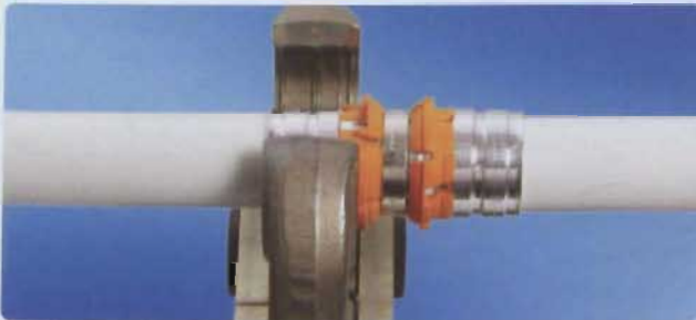
Positioning : the jaws are fitted up to the stop ring
