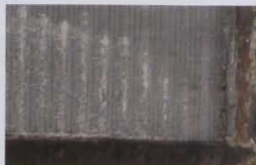
After a 5000 hour salt mist/ ammonium sulphate test the image above shows a traditional coil whilst the image below shows a MCHX coil
