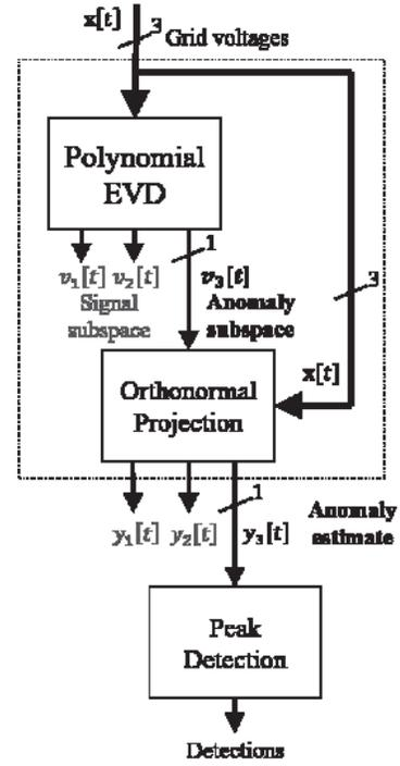
**Fig. 1** Block diagram representation of the proposed approach, where the system blocks outlined by the dotted box constitute broadband subspace decomposition.
