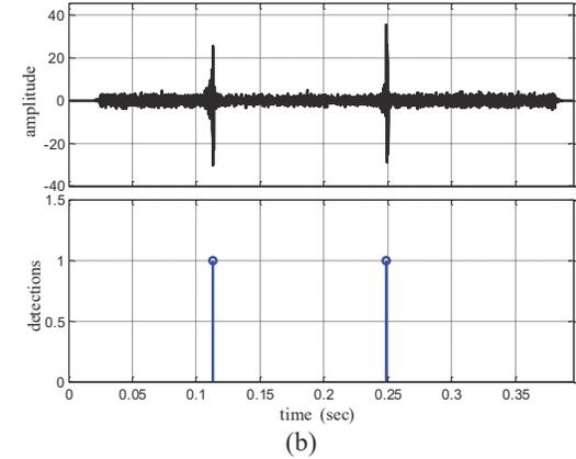
Fig. 3 Performance of the proposed system under three-phase voltage sag condition (a) captured results in oscilloscope (b) determined faulty interval.
