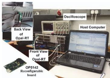
Fig. 2 Real-time laboratory set up with OPAL-RT.
