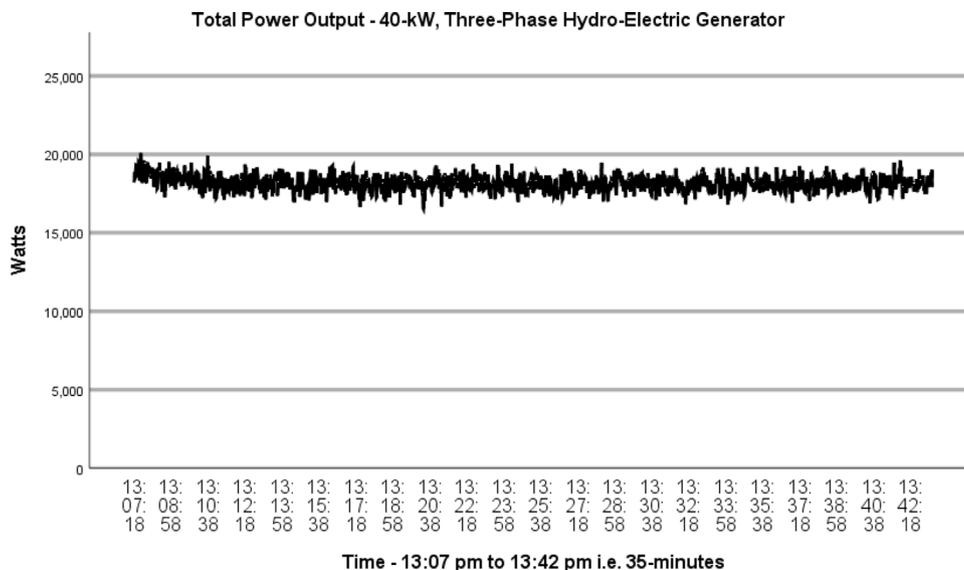
Fig. 7. Hydroelectric power output over 35-min, half-second sampling time (Kealy, 2020).
