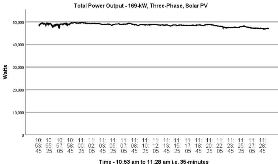
Fig. 6. Solar PV power output over 35-min, half-second sampling time.
