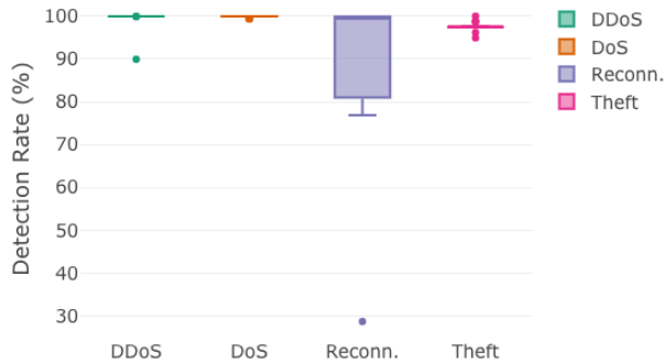
Fig. 3. Boxplots show the distribution of each unknown attack detected by GE algorithm (each boxplot represents an experiment of 20 independent runs).
