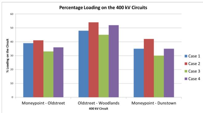
Figure 6 - Percentage loading on the 400 kV circuits
