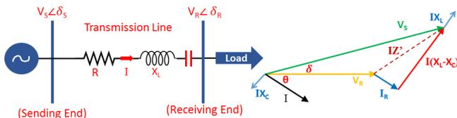
Figure 1 - Series compensation on a transmission line
