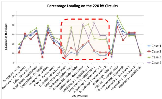
Figure 7 - Percentage loading on the 220 kV circuits
