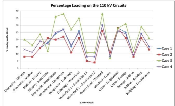
Figure 8 - Percentage loading on the 110 kV circuits
