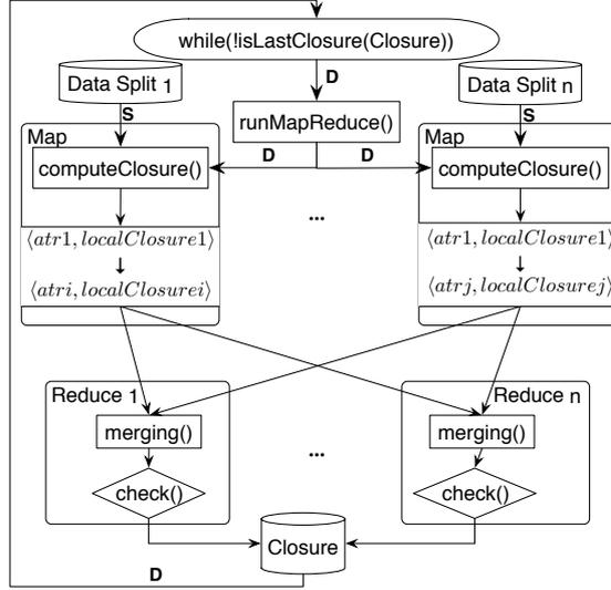
**Fig. 1.** MRGanter work flow: static data is loaded at the start of the procedure (labeled by S) and the dynamic data (closures produced during each iteration) is passed and used in the next iteration (labeled by D).
