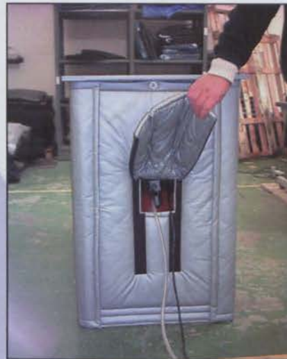
Mobile compressor enclosure with attenuated air inlet and hose/cable outlets
