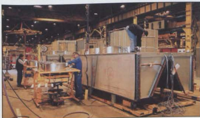
Chiller manufacturing at the Trane ISO 9001-accredited factory in Cluses, France.
