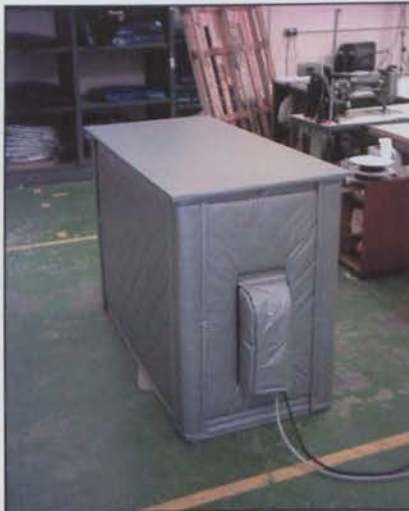
Compressor enclosure incorporates solid worktop lid (chequered plate option)
