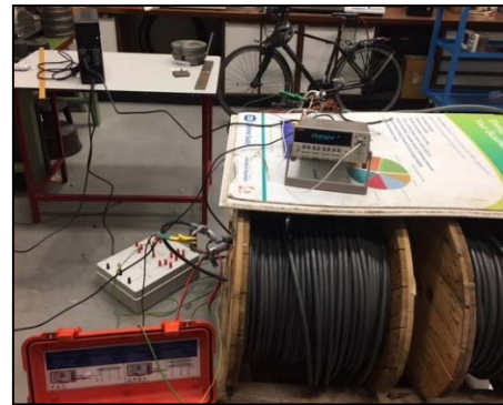
Fig. 2. Nanovoltmeter and Fault Location Device – Volt Drop Measurement
