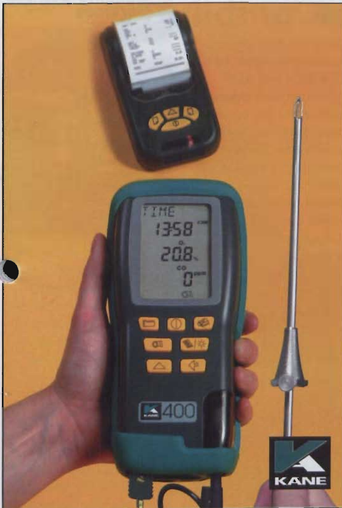
If you mainly service oil or larger gas boilers, a full flue gas analyser such as the popular Kane 400 is recommended.
