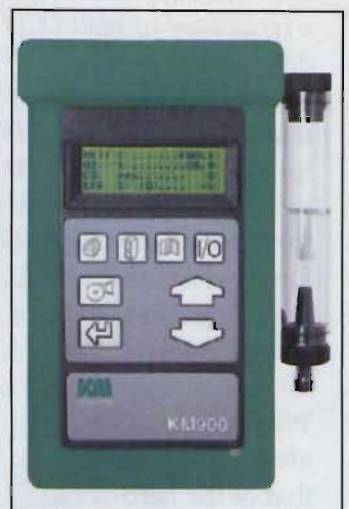
Models such as the KM900 can also measure NO x and download to a PC
