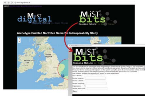
Fig. 4. The OPTaaS backend infrastructure is implemented as a set of RESTful [40] Web services using Groovy/Grails [41] and Java [42]. New platforms can register against community agreed archetypes/opts where the platform then receives a micro-context template to constrain their observational data
