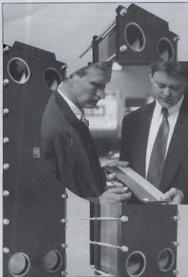
SWEP's heat exchangers use thin plates of high thermal conductivity, pressed into meticulously-calculated herringbone patterns. Details from Eurofluid Handling Systems.
