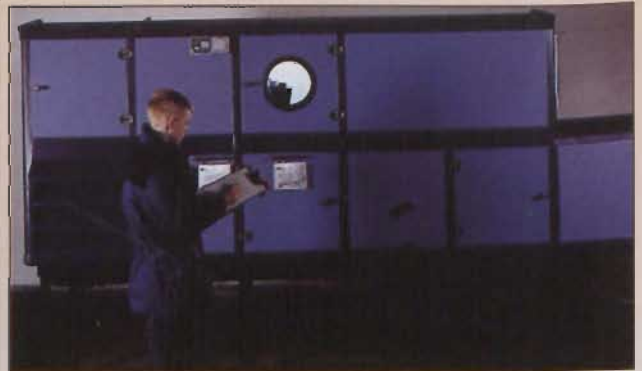
Quality control inspector examining a frameless air conditioning unit as it comes off Masterair's manufacturing line
