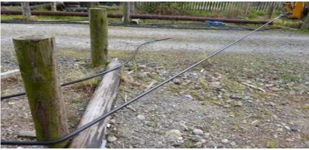
Fig. 2. Sidewall Loading Test - Cable sample is experiencing a tensile strain and sidewall force at the 75° bend angle
