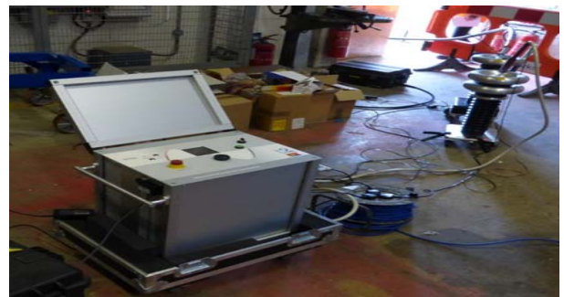
Fig. 4. Partial Discharge and Tan \delta Test - Mechanically stressed cables undergo high voltage defects diagnostic tests
