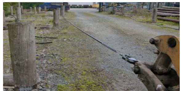
Fig. 1. Tensile Strain Test - Three cable samples were pulled to different tensile strains i.e. 700 kg, 1500 kg and 2000 kg
