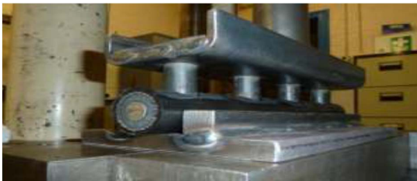
Fig. 3. Compressive Force Test - Rig designed so all force transmitted to the conductor via vertical prongs having drilled the cable at intervals
