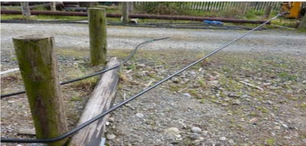
Fig. 2. Sidewall Loading Test - Cable sample is experiencing a tensile strain and sidewall force at the 75° bend angle
