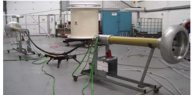
Fig. 7. Test arrangement in PowerCSL - Four times the nominal voltage applied to cable samples for four hours during Noise Free PD test
