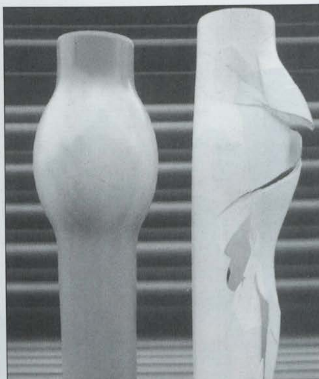
Aquaforce from Uniplas offers high ductility and shatter resistance. Left: Aquaforce; Right: Conventional uPVC.
