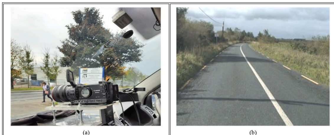
Fig. 1. Typical camera position, captured image, and the image after different pre-processing steps. (a) is the picture of a typical camera position mounted on the video van. (b) the output of the camera with a rating of 10.
