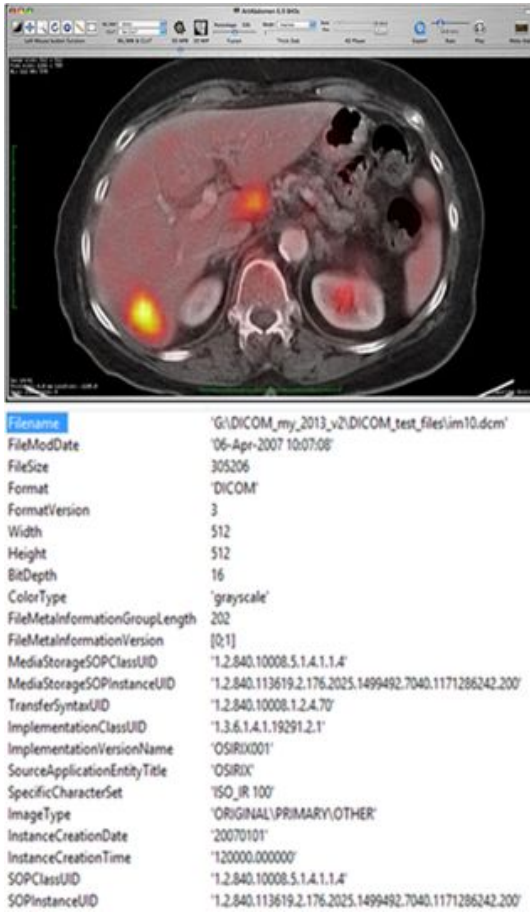
Fig. 1: Example DICOM image viewed using OsiriX [1] (above) and some example DICOM Metadata (below).
