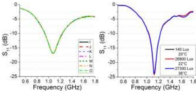
Fig. 6 – Reflection Coefficient Variation of Full Solar Antenna
