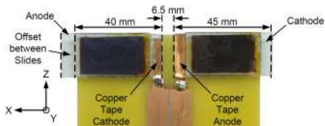
Fig. 1 – Rear of dye-Sensitised Solar Dipole Antenna
