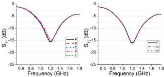
Fig. 4 – Reflection Coefficient Variation of ITO Antenna
