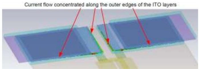
Fig. 8 – Current Flow on Full Solar Antenna
