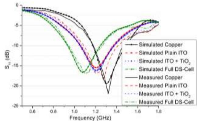
Fig. 3 – Measured and Simulated S<sub>11</sub> Results
