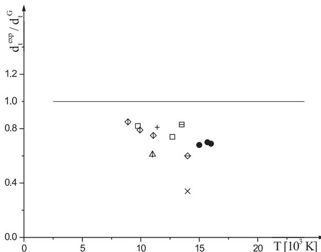
Fig. 2. Ratios of the experimental total shift ( $d_t^{\text{exp}}$ ) to the theoretical ( $d_t^{\text{G}}$ ) predictions [26] vs. electron temperature for  $\lambda=425.936$  nm. ●, our experimental results and those of other authors:  $\square$ , Ref. [15]; +, Ref. [16];  $\times$ , Ref. [17];  $\triangle$ , Ref. [18];  $\phi$ , Ref. [19];  $\diamond$ , Ref. [24] and  $\square$ , Ref. [25].
