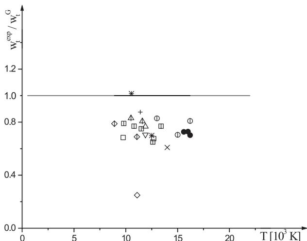
Fig. 1. Ratios of the experimental total Stark FWHM ( $W_t^{\text{exp}}$ ) to the theoretical ( $W_t^{\text{G}}$ ) predictions [26] vs. electron temperature for  $\lambda=425.936$  nm. ●, our experimental results and those of other authors:  $\Delta$ , Ref. [12];  $\nabla$ , Ref. [13];  $\diamond$ , Ref. [14];  $\square$ , Ref. [15]; +, Ref. [16];  $\times$ , Ref. [17];  $\triangle$ , Ref. [18];  $\phi$ , Ref. [19]; \*, Ref. [20];  $\odot$ , Ref. [22] and  $\square$ , Ref. [23].
