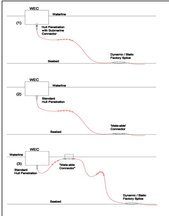
**Fig. 4:** Dynamic / Static Cable Connection Options for WEC
