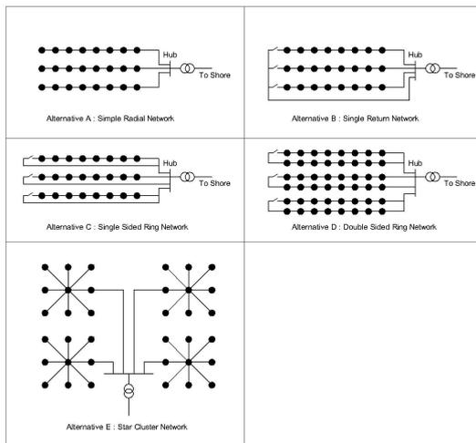
Fig. 1: Alternative Array Network Configurations
