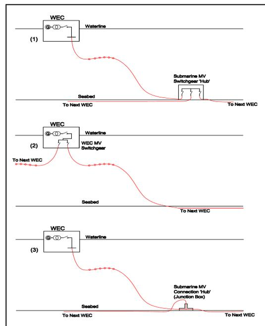
**Figure 5:** Switchgear Options for Floating WEC
