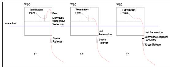
Fig. 3: Dynamic Cable / WEC interface options for WEC
