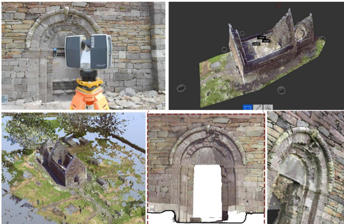
Figure 2. Faro Terrestrial Scan of Kilmalkeader Romanesque Church (Discovery Programme), the top left image shows the Faro scanner used the top left image illustrates the processed point cloud and the bottom images illustrate the unprocessed and registered scan on the left and in contrast the use of photogrammetry to capture the doorcase.
