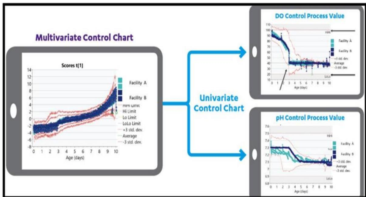
Figure 3: Model used at Facility A to support Tech Transfer of product to Facility B. Multivariate Control chart demonstrates that both facilities perform similarly in batch production (reproduced with permission – see reference 2)
