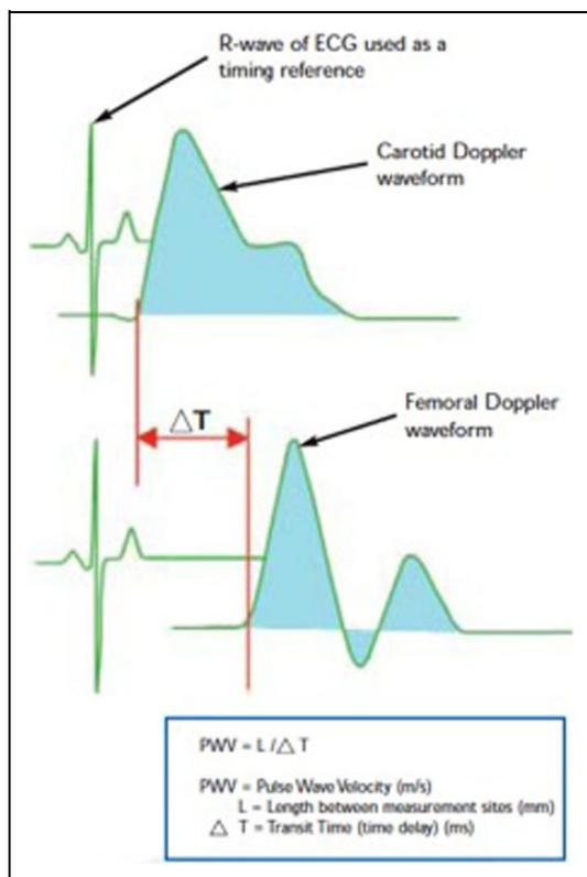
**Figure 3.** Measurement of PWV using the R-wave of the ECG trace as a timing reference. PWV indicates pulse wave velocity; ECG, electrocardiogram.
