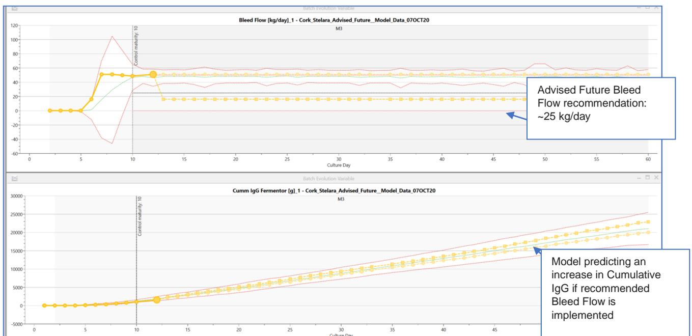
**Fig 1: Advised Future Model advising to adjust bleed rate of bioreactor within its specification range to increase total amount of product output.**
