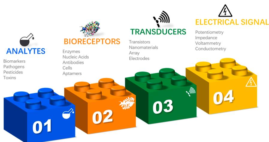
**Figure 1.** Simplified components' representation of an electrochemical biosensor.
