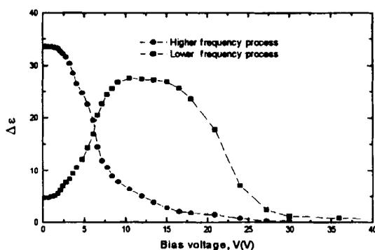
FIGURE 2. Dependence of the dielectric strength on the bias voltage for AS-573,  $d=50 \mu\text{m}$ ,  $T=86^\circ\text{C}$ .  $\bullet$  - ferrielectric relaxation,  $\blacksquare$ - ferroelectric relaxation.
