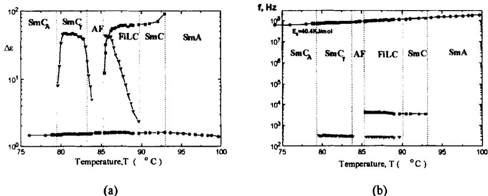
FIGURE 1. Dependence of the dielectric strength (a) and relaxation frequency (b) on temperature for AS-573,  $d=50 \mu\text{m}$ . ●-β- relaxation around long axis, ■- ferroelectric and ▼ - ferrielectric Goldstone modes.
