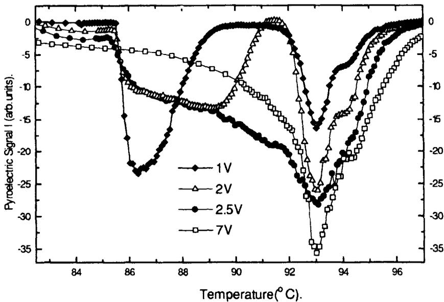
FIGURE 2 The Pyroelectric Signal  $I$  (arbitrary units) versus Temperature ( $^{\circ}\text{C}$ ) for bias voltages of  $V=1, 2, 2.5, 7 \text{ V}$ . The pyroelectric signal shown for  $7 \text{ V}$  is divided by 3.
