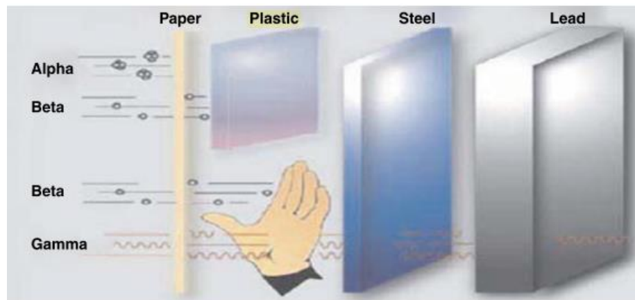
Figure 1.3 Various ionising radiation penetration ranges. Electrons have smaller ranges and travel shorter distances than gamma and X-rays, and they can be absorbed by plastics, glass and metal layers (Internal Atomic Energy Agency Publications, IAEA 2004).
