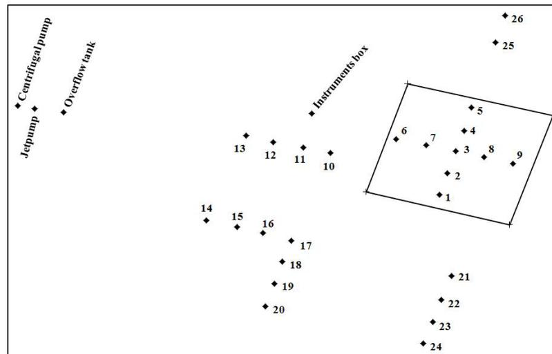
**Figure 4** – Surface settlement plates and stand pipes distribution
