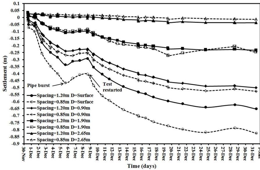
Figure 5 – Ground settlement at different depths for both spacing subareas
