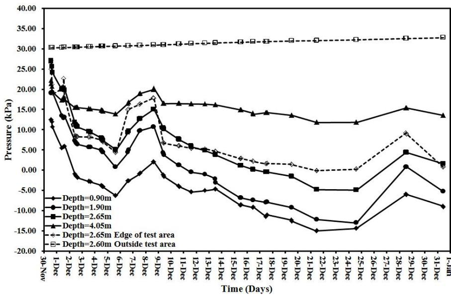
Figure 6 – Pore-water pressure variation for 0.85m PVD spacing subarea
