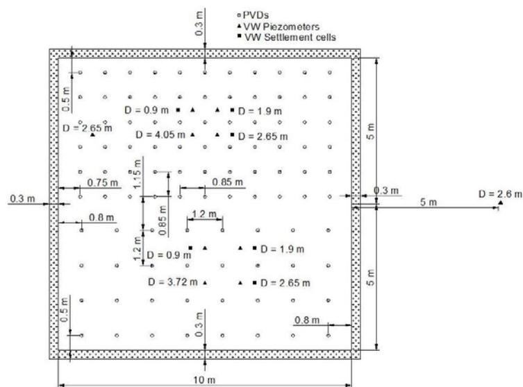
**Figure 2** - PVD and subsurface instrumentation arrangement
