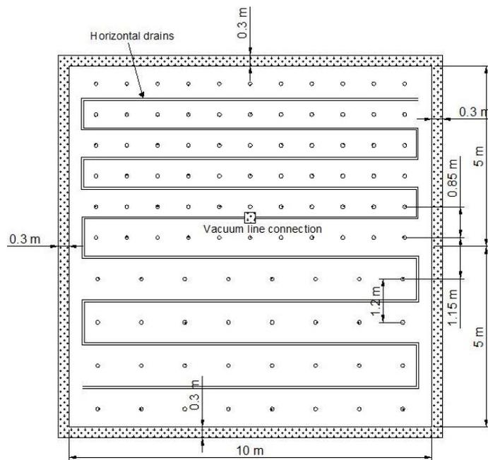
**Figure 3** - Horizontal drains arrangement
