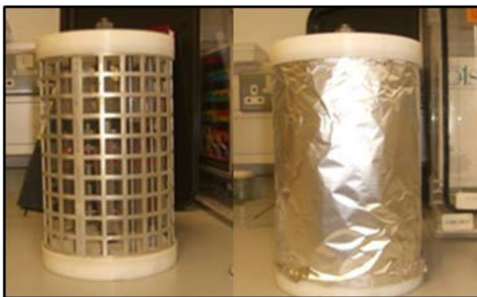
Figure 5.2 The SPMD and PDMS Cage containing the samplers which was covered in aluminium to protect against air borne particles/contamination during deployment.
