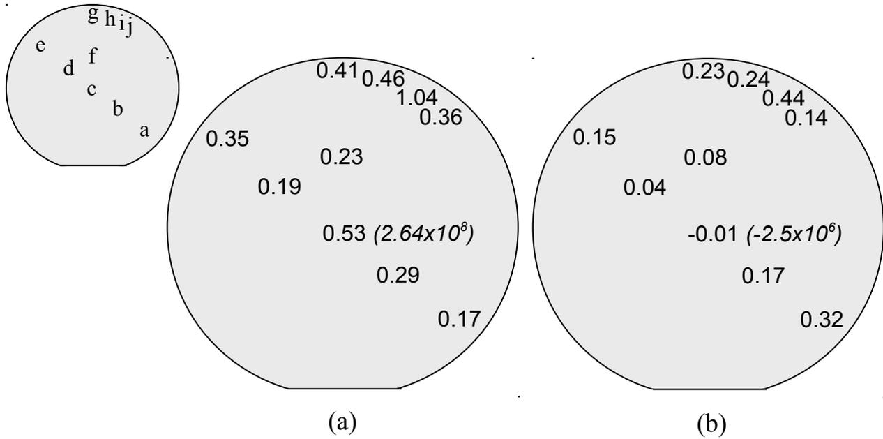
Fig. 4. Raman peak shift measurements ( $\Delta\omega$ ) for (a) Wafer A: RTD at 1000 °C for 15 s, (b) Wafer B: RTD at 1000 °C for 165 s. A positive shift in the Raman peak position corresponds to a compressive stress, and a negative shift corresponds to a tensile stress. The value in brackets denotes the stress,  $\sigma$ , (in Pa), calculated using equation 2.
