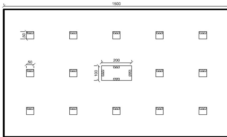
**Figure 1.** Front elevation of the lighting booth. Note the smaller measuring hatches and the larger central hatch for viewing. Measuring hatches, at similar spacing, were used on all sides of the booth, including the top and bottom surfaces.
