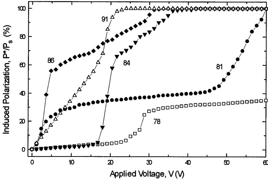
FIG. 9. Temperature dependence of the normalized spontaneous polarization as function of bias voltage for different phases: Sm- $C^*$ , 91 °C; FiLC, 86 °C; AF 84 °C; Sm- $C_\gamma^*$ -81 °C; Sm- $C_A$ , 78 °C. The cell thickness is 50  $\mu\text{m}$ .
