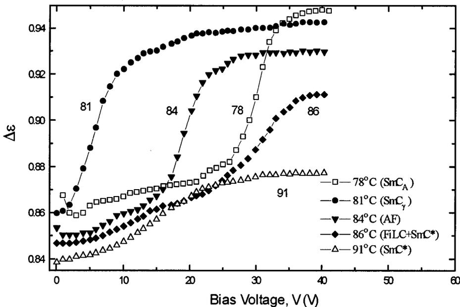
FIG. 10. Temperature dependence of the dielectric strength of the high-frequency molecular relaxation as function of bias voltage for different phases: Sm- $C^*$ , 91 °C; FiLC, 86 °C; AF, 84 °C; Sm- $C_\gamma^*$ , 81 °C; Sm- $C_A$ , 78 °C. The cell thickness is 50  $\mu\text{m}$ .
