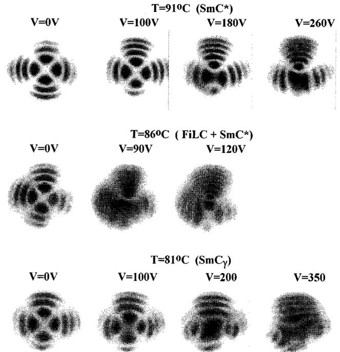
FIG. 2. Conoscopic pictures under bias voltage different phases: Sm- $C^*$ ,  $91^\circ\text{C}$ ; FiLC,  $86^\circ\text{C}$ ; Sm- $C_\gamma$ ,  $81^\circ\text{C}$ .
