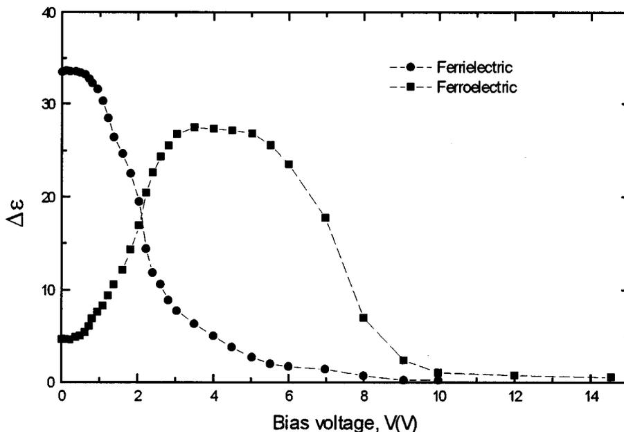
FIG. 8. Dielectric strength vs bias voltage for the low-frequency (ferrielectric) relaxation process and higher-frequency (ferroelectric) relaxation process at  $T=86^\circ\text{C}$ . The cell thickness is 50  $\mu\text{m}$ .
