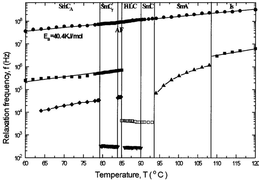
FIG. 4. Dependence of the relaxation frequency ( $f$ ) on temperature for AS-573  $d=50 \mu\text{m}$ ; the temperature range is divided up into the various phases.
