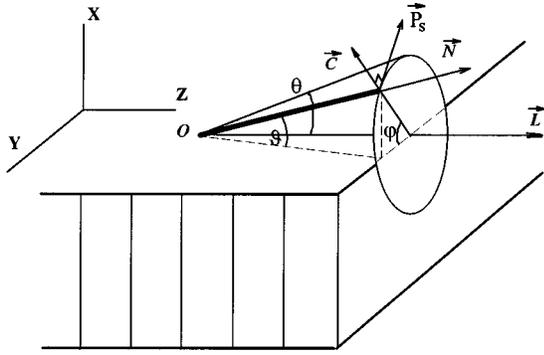
FIG. 6. Smectic layer structure for a bookshelf cell.  $(X, Y, Z)$  is the coordinate system,  $N$  is the molecular director,  $L$  is the smectic layer normal,  $C$  is the  $c$  director,  $\theta$  is the tilt angle,  $\vartheta$  is the angle between molecular director and the electrode plane, and  $\varphi$  is the azimuthal angle; the plane  $YZ$  is that of the glass plate.
