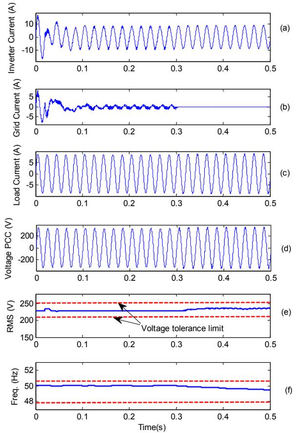
Fig. 7. Case of “close to zero” power mismatch (NDZ) with passive method
