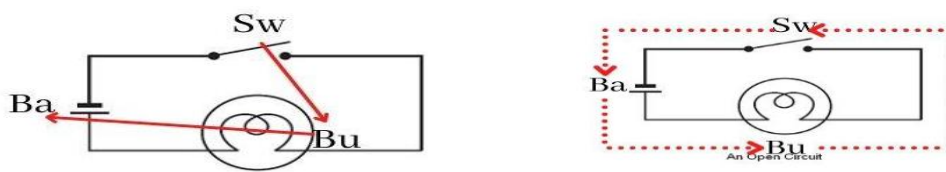
Fig. 2: Novice's (left) and expert's (right) order of attention for circuit 1. The straight arrows indicate attention to elements such as switch, bulb and battery. The dotted line indicates attention to elements based on the direction of the current.
