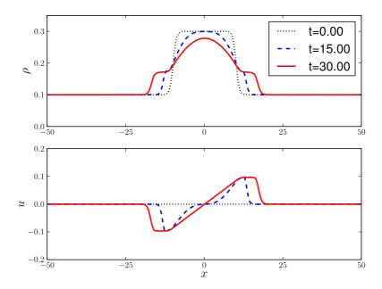
Figure 2: Dam-break results for the system (7)-(8) shows evolution of the elevation  $\rho$  (upper panel) and velocity u (lower panel), arising from initial conditions (10)-(11) in a periodic domain. observe a wave with a slope that is becoming closer to vertical which eventually forms a breaking wave. Figures are courtesy of J. Percival.
