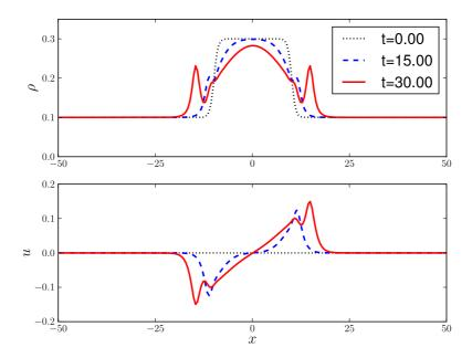
Figure 1: Dam-break results for the CH2 system in equations (2)-(3) show evolution of the elevation  $\rho$  (upper panel) and velocity u (lower panel), arising from initial conditions (10)- (11) in a periodic domain. The soliton solutions are seen to emerge after a finite time, and the evolution of both variables generates more and more solitons propagating in both directions as time progresses. Figures are courtesy of J. Percival.
